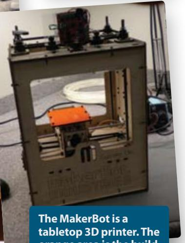
The MakerBot is a tabletop 3D printer. The orange area is the build platform.
