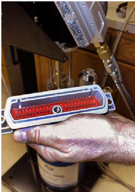
Applying contact lubricants on the automotive assembly line usually is limited to injecting grease or dipping in a dispersion. The process can be automated to minimize operator involvement.
